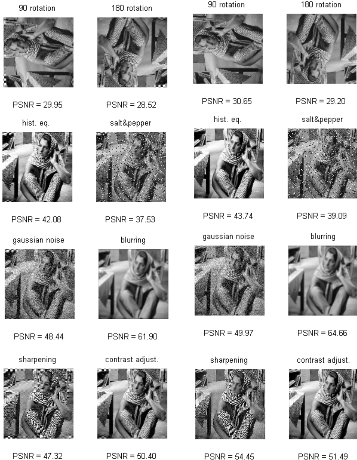
Fig. 3-a-DWT-SVD attacked watermarked images and their PSNR values
